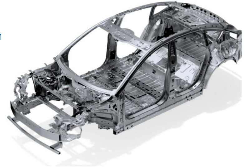
ET5's single-piece casting
