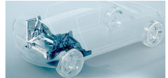
Volvo's Mega Casting process for aluminum body parts
