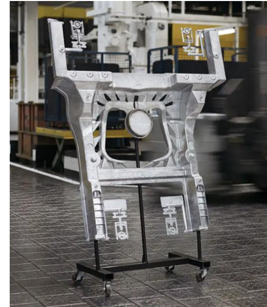
VW will use the megacasting equipment at its factory in Kassel
