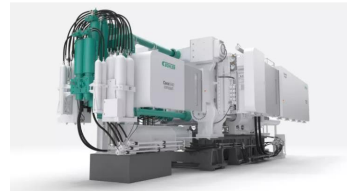
Volvo's Mega Casting process for aluminum body parts
