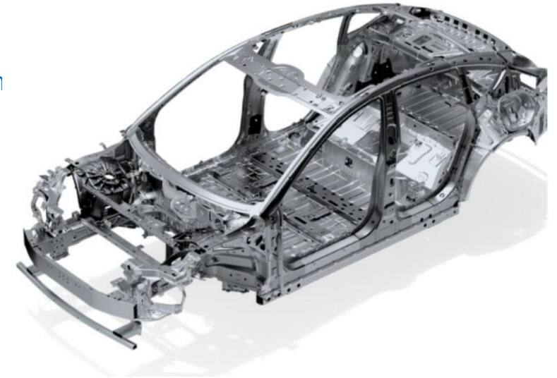
ET5's single-piece casting
